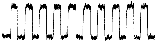
Figure 9. Signals obtained for Pb 4057.8 Å for a solution containing 0.2 µg/ml Pb. Analyte and blank solutions were run alternately at 1-minute intervals
